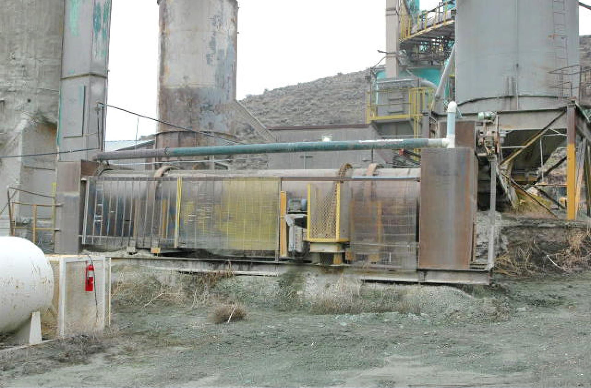
**Dryer feed bin on right for Raymond mill and liners 1 and 2 for granular products.**
