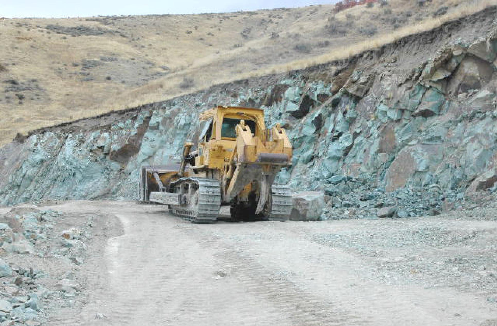
Face of zeolite in front of D8K with ripper.
