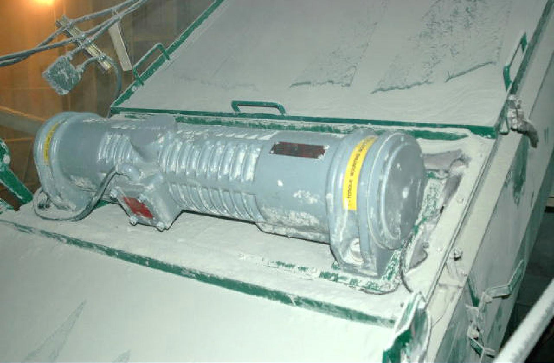
Derrick 3600rpm high frequency screen for line one.
