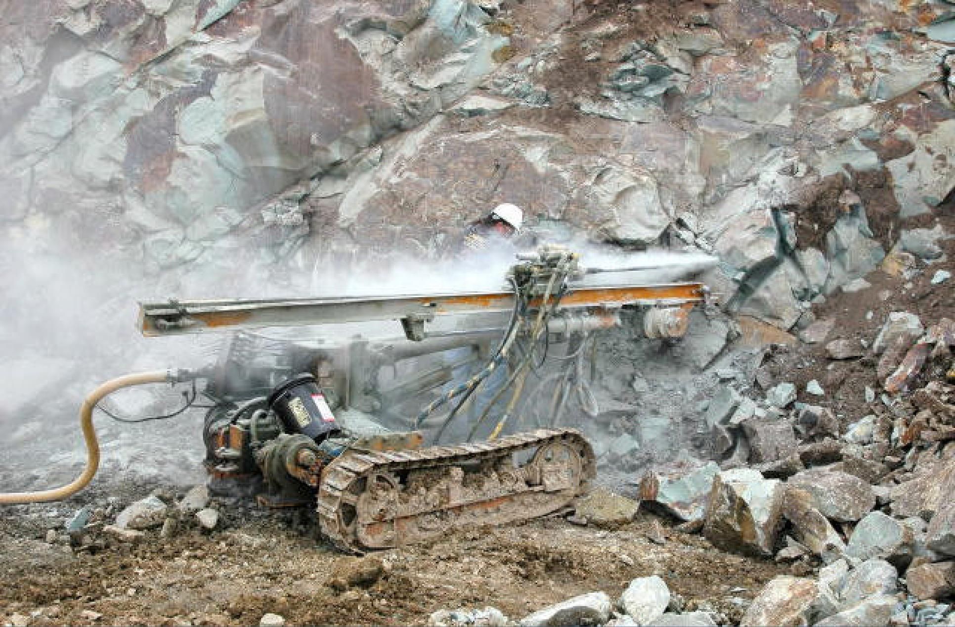
**Blowing blast hole air track.**
