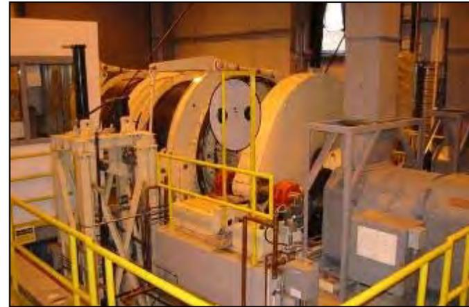
**8' diameter Nordberg Hoist at Vent Shaft–
