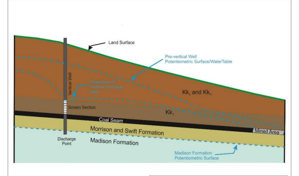
Conceptual Cross Section for Vertical Well Design
