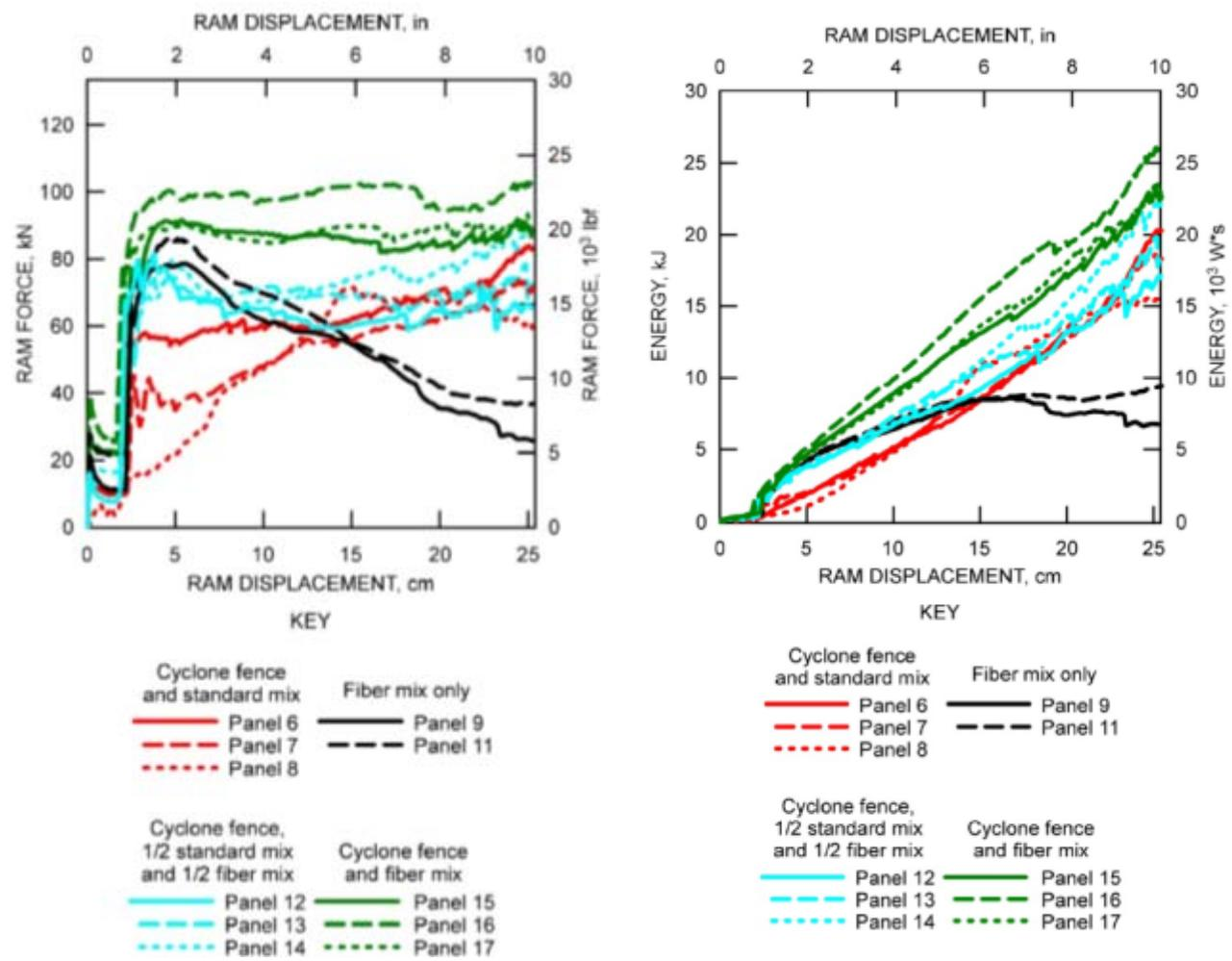
Note: Test results primarily show energy dissipation of the shotcrete/chain link as D-Bolts not failed.
