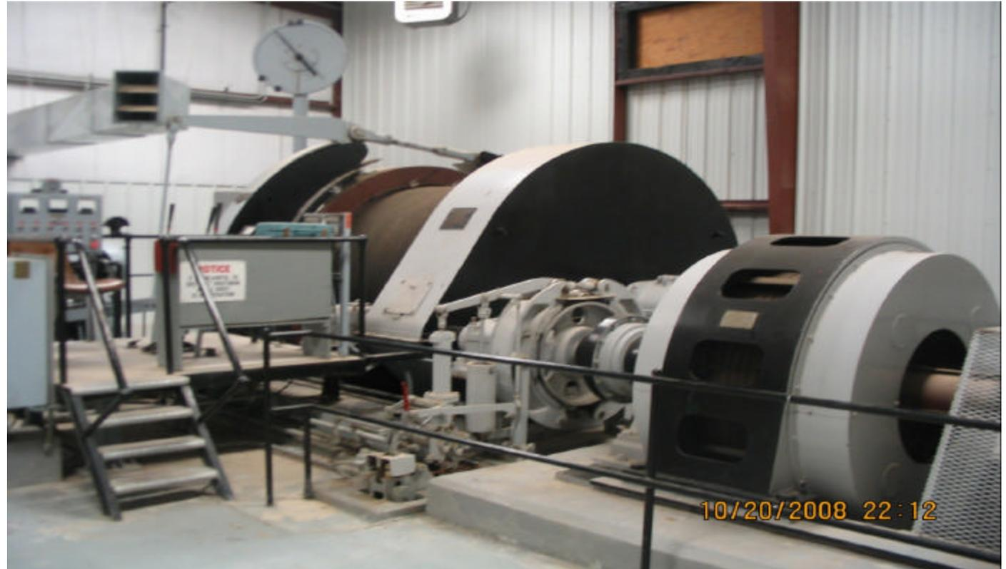
Hoist Capacity - 80 tons/hr
