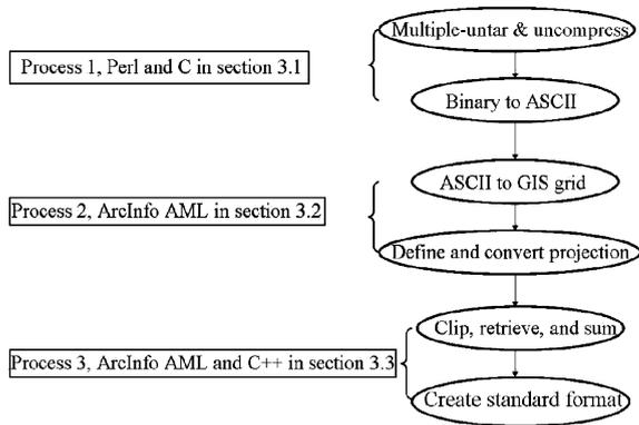
Fig. 1. Work flow chart showing entire automated processes by using commercial GIS and a number of Perl scripts and C/C++ programs.
