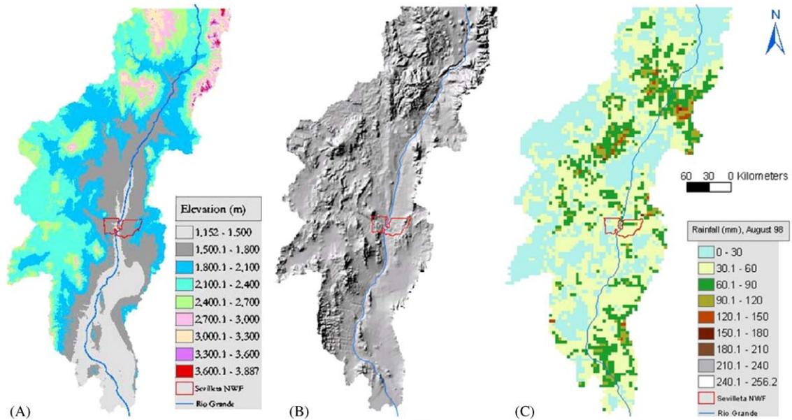
Fig. 5. DEM (A), shaded relief DEM (B), and NEXRAD precipitation (C) of August 1998 in the Upper Rio Grande Basin within New Mexico are readily for various GIS spatial and statistical analyses or input for hydrologic modeling.
