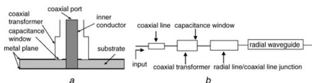
Fig. 2 Equivalent-circuit model of current probe circuit
