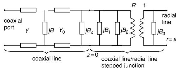
Fig. 3 Equivalent circuit of current probe circuit
