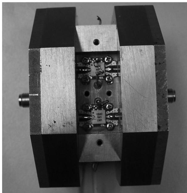
**Figure 8** A picture of the radial waveguide power amplifier fabricated
