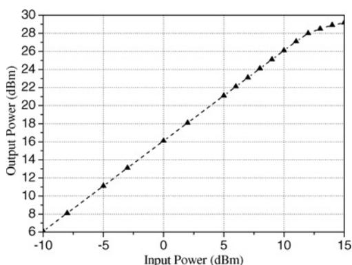
Figure 10 Output power against input power of the eight-device power amplifier at 10 GHz
