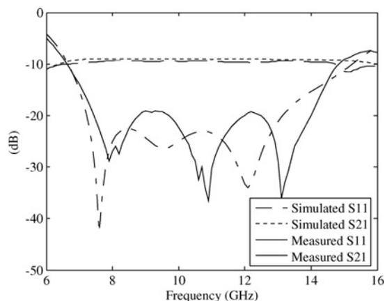
**Figure 7** Simulated and measured  $S$ -parameters of the power divider
