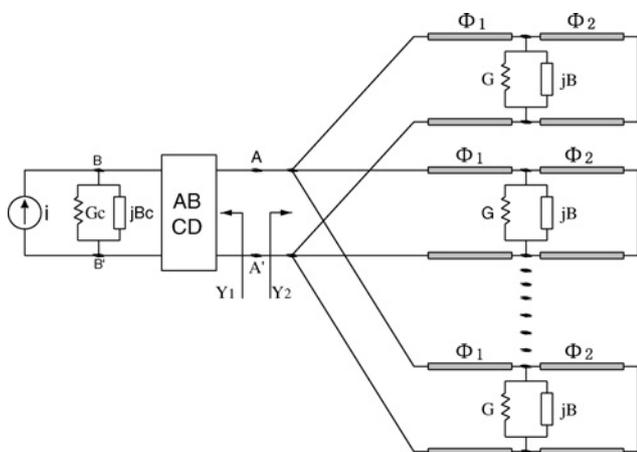
**Figure 5** An equivalent circuit of the  $N$ -way radial waveguide power divider
