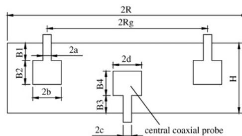
**Figure 2** Topology of a radial waveguide power divider
