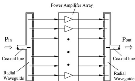
**Figure 1** A schematic of the radial waveguide power combiner
