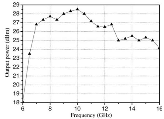
Figure 11 Measured  $P_{out}@1$  dB of the eight-device power amplifier
