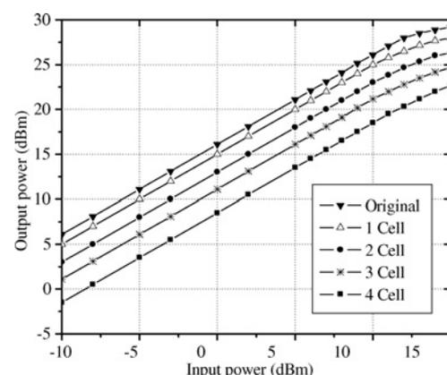
Figure 12 Measured output power drops as various numbers of device failures
