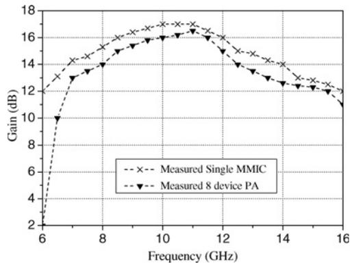
Figure 9 Measured small-signal gain
