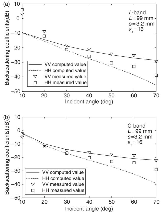
Figure 3. Comparisons of the model predictions (lines) with measurements (symbols) from a bare soil surface 30% surface moisture at (a) 1.515 GHz and (b) 4.725 GHz.
