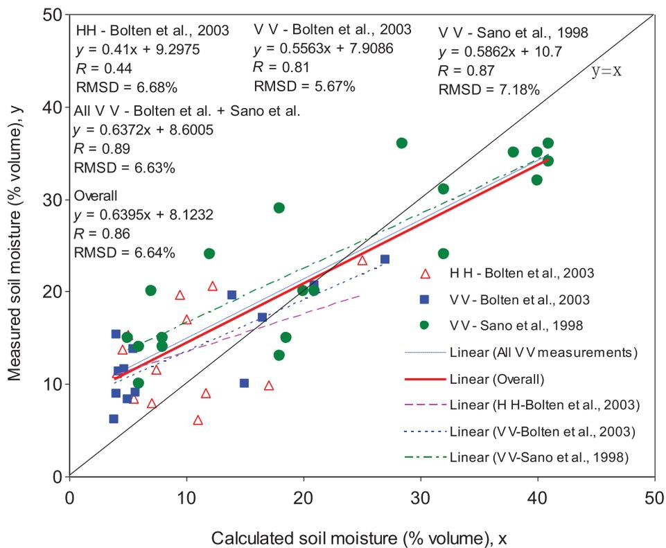
Figure 4. Correlation between the soil moisture contents calculated by the inversion algorithm and those measured by Bolten et al.[2] and Sano et al.[8].
