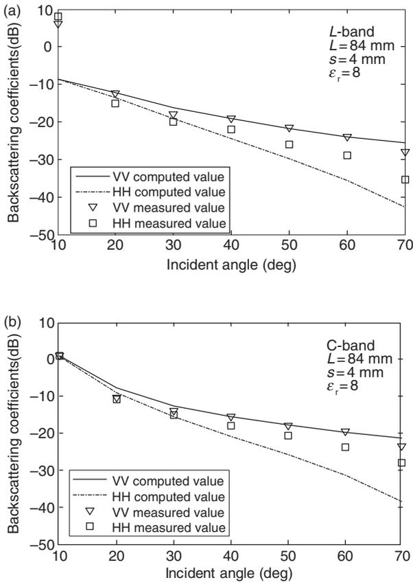
Figure 2. Comparisons of the algorithm predictions (lines) with measurements (symbols) from a bare soil surface 14% surface moisture content at (a) 1.515 GHz and (b) 4.725 GHz.
