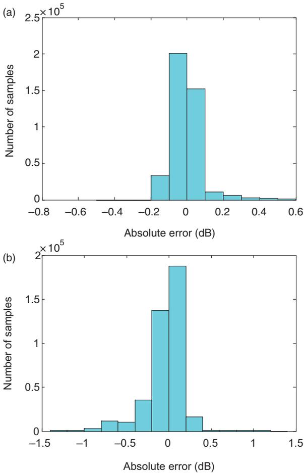
Figure 1. Histogram of absolute error in dB between the SPM model and the SPM fitting algorithm for (a)  $\sigma_{hh}$ ; and (b)  $\sigma_{vv}$ . The total number of samples is 408,000.
