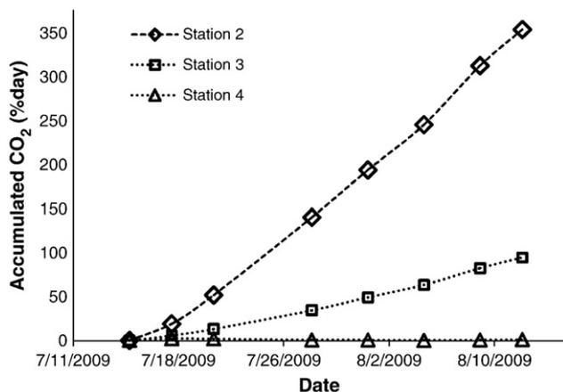
Fig. 2. Accumulated soil CO<sub>2</sub> concentration (%day) during the CO<sub>2</sub> injection experiment. Instantaneous soil CO<sub>2</sub> concentration ranged 0.6–19% for station 2 and 1–6.5% for station 3. For station 4, soil CO<sub>2</sub> concentration was almost stable (1.5–1.0%), indicating background normal soil CO<sub>2</sub> levels.
