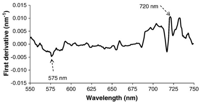
Fig. 7. The typical first derivative of reflectance with respect to wavelength of mixed vegetation on 7/18/2009 at station 2 of the transect. The arrows indicate the positions of local extremes used to generate normalized difference first derivative index (NFDI).
