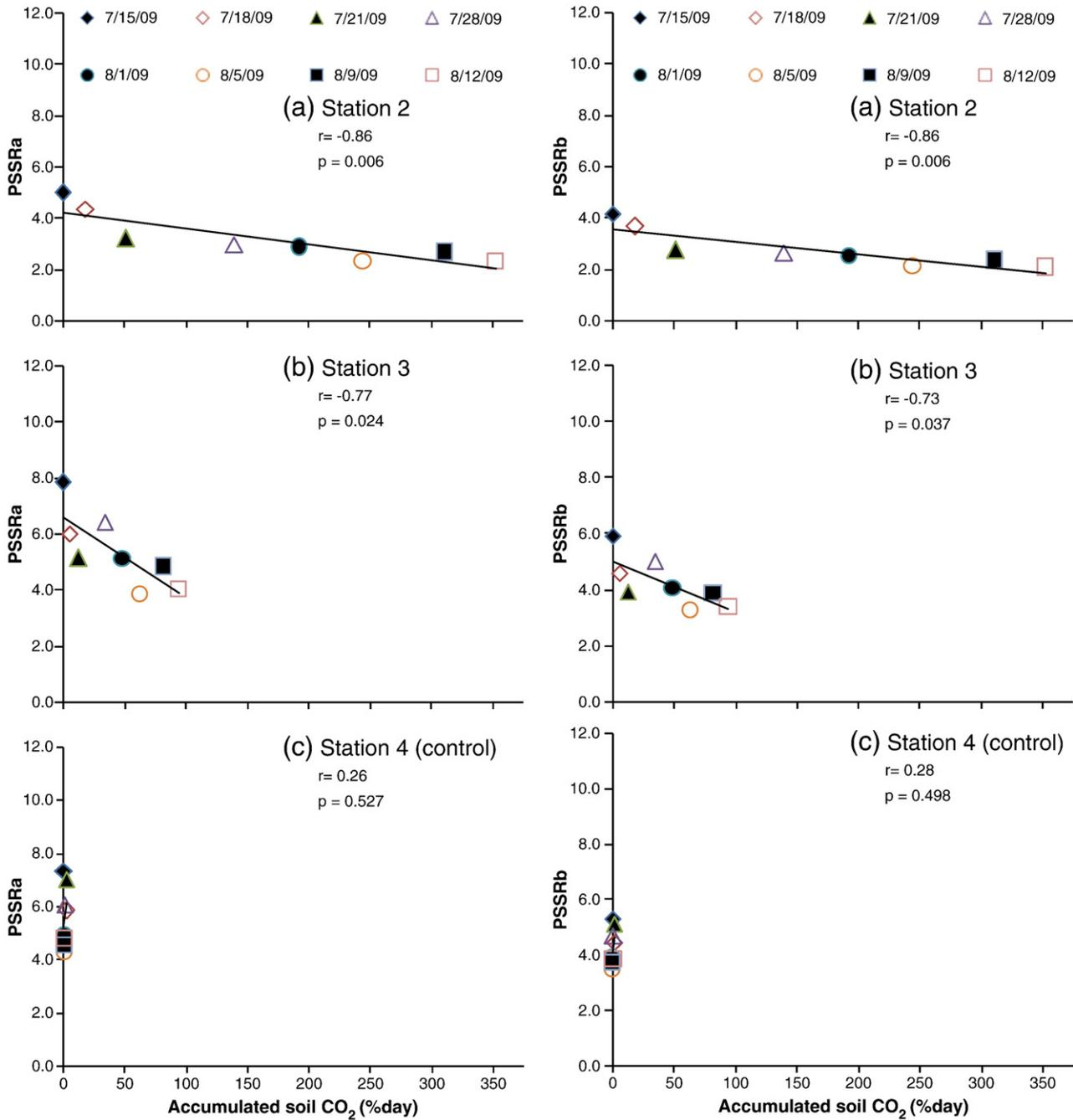
**Fig. 6.** Both PSSRa and PSSRb have negative linear trends at stations 2 and 3, indicating a decrease in chlorophyll *a* and chlorophyll *b* concentration with increasing levels of soil CO<sub>2</sub>. At station 4, the correlation shows a poor relationship with soil CO<sub>2</sub> and thereby indicates natural growth of vegetation at this site was unaffected by the leaking CO<sub>2</sub>. Dates of data collection and corresponding symbols are indicated in (a).
