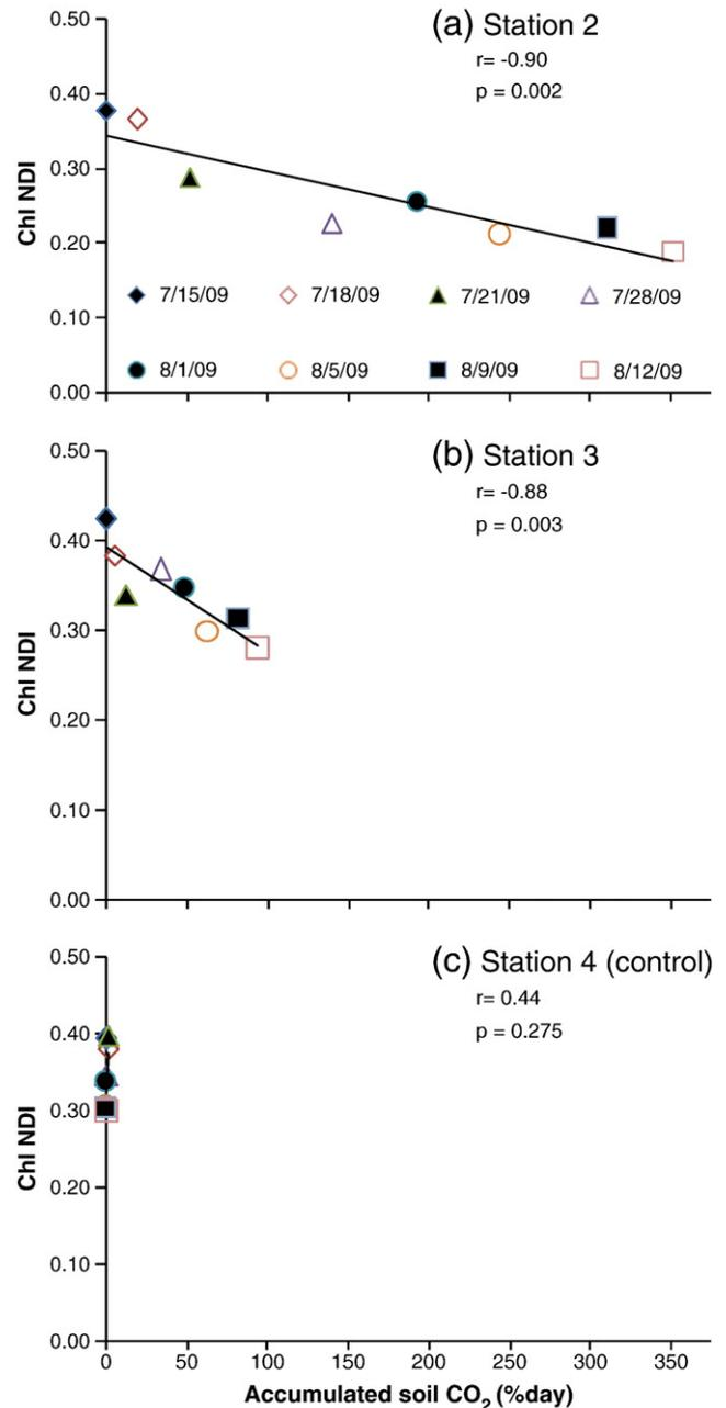
**Fig. 5.** Scatter plots indicating the relationship between chlorophyll normalized difference vegetation index (Chl NDI) and accumulated soil CO<sub>2</sub> for (a) stations 2, (b) station 3, and (c) station 4. The negative correlation at stations 2 and 3 was due to a decrease in chlorophyll content of leaves and the positive correlation at station 4 indicates no effect of CO<sub>2</sub> leakage. Dates of data collection and corresponding symbols are indicated in (a).
