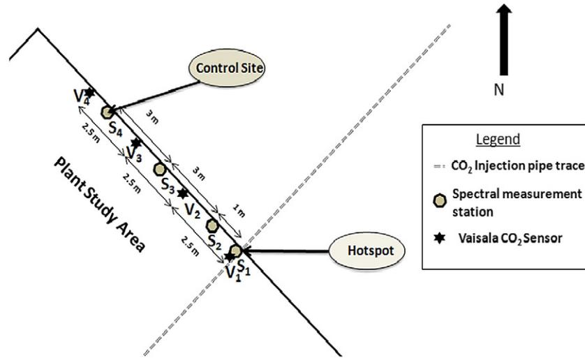
**Fig. 1.** Schematic diagram of the plant study area at the ZERT field facility for the summer 2009 shallow CO<sub>2</sub> release experiment. The transect was divided into 4 stations (S<sub>1</sub>–S<sub>4</sub>, shown by circles) with station 1 being on the injection pipe and station 4 approximately 7 meter away from the pipe. Stars indicate the locations of soil CO<sub>2</sub> concentration probes (V<sub>1</sub>–V<sub>4</sub>). The distance between S<sub>1</sub> and V<sub>1</sub> was 0.25 m.
