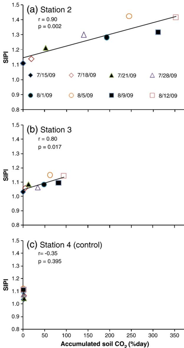
**Fig. 4.** Correlation between structural independent pigment index (SIPI) and accumulated soil CO<sub>2</sub> percent data for: (a) station 2 and (b) station 3, positive correlations ( $r = 0.90$  and  $r = 0.80$ ) indicates an increase in carotenoids/chlorophyll *a* concentration, (c) Station 4, correlation ( $p = 0.395$ ) is not significant at 95% level, indicating no effect of leaking CO<sub>2</sub>. Dates of data collection and corresponding symbols are indicated in (a).
